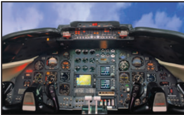
The Honeywell/West Star Aviation RVSM Solution for Learjet 30-series aircraft — STC awarded July 3, 2003. The company has also developed an RVSM solution for Conquest II aircraft with the Meggitt MAGIC® or APS-65 autopilot installed
